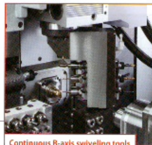
Continuous B-axis swiveling tools Frontal rotary tool: 3 (Collet ER/AR16) Back rotary tool: 3 (Collet ER/AR11)
